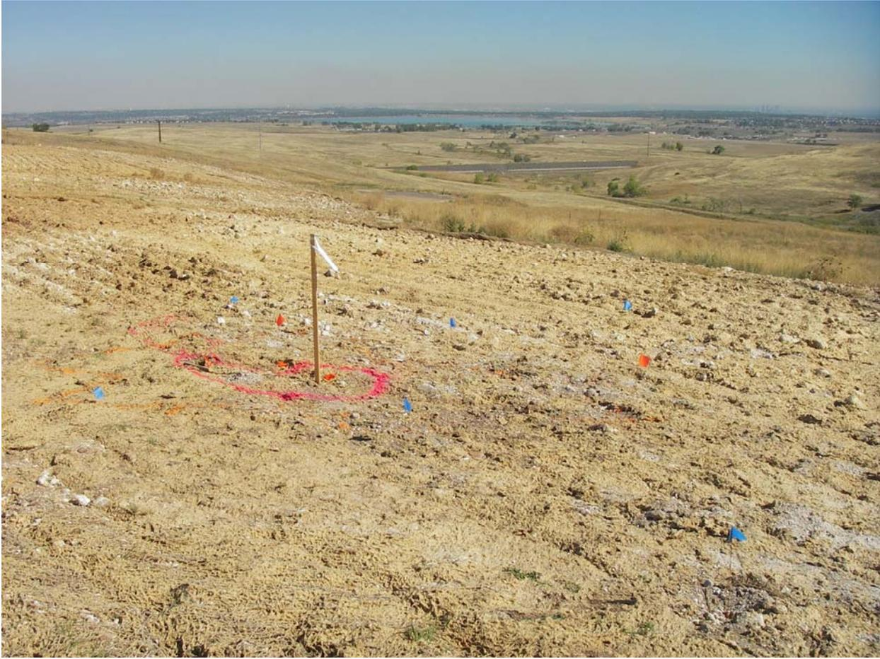
**Figure 4. Close-up of Pu hotspot shown in Figure 3 (red spray paint marks hotspot boundary). This hotspot along with 12 others found by ORISE were remediated to below the 50 pCi/g WRW AL for Pu**
